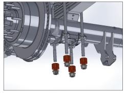
Reinstall factory U-bolts with the supplied **Axle U-bolt Spacers** between the axle cradle and the U-bolt nuts.
