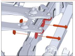
First remove the 5th wheel frame mounting hardware.
