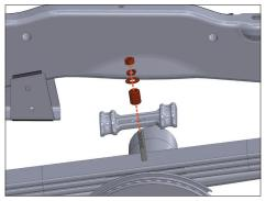
Reinstall the factory U-bolt saddle and install the supplied **Center Pin Spacer** with the correct size flat washer, split washer, and factory center pin nut.
