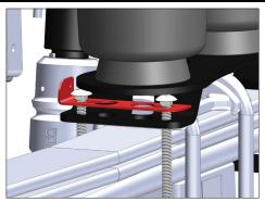
When attaching the lower air spring bracket, install the height sensor relocation bracket between the carriage bolts and the lower bracket leg.
