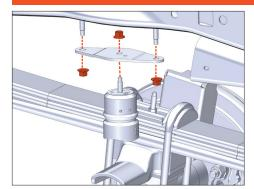
Unbolt factory bumpstop using a 15MM socket.
