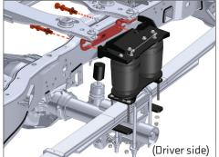
Use the supplied 4" long Grade 8 5/8" bolts, Repeat for passenger side. with split washers and flat washers, to attach the upper air spring bracket to the outside of the hitch, through the factory hitch mounting holes. Snug hardware.
