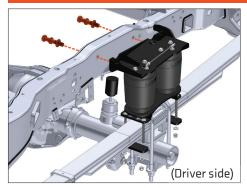
Use the supplied **3.5"** long Grade 8 5/8" bolts, Repeat for passenger side. with split washers and flat washers, to attach the upper air spring bracket to the outside of the frame, through the factory sleeved holes. Snug hardware.
