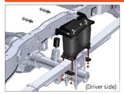
Use the supplied 3/8" hardware and leaf spring straps to attach the lower air spring bracket to the leaf spring.
