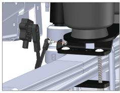
Attach the height sensor linkage arm to the relocation bracket using the factory nut.
