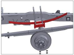
Spray the factory center pin nuts and axle U-bolt nuts with penetrating oil.
