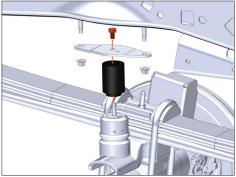
Reinstall factory bumpstop with provided Repeat for passenger side. aluminum spacer and M10 bolt.
