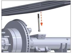
Remove the factory center pin from the leaf pack by driving it out from the top with a punch.
